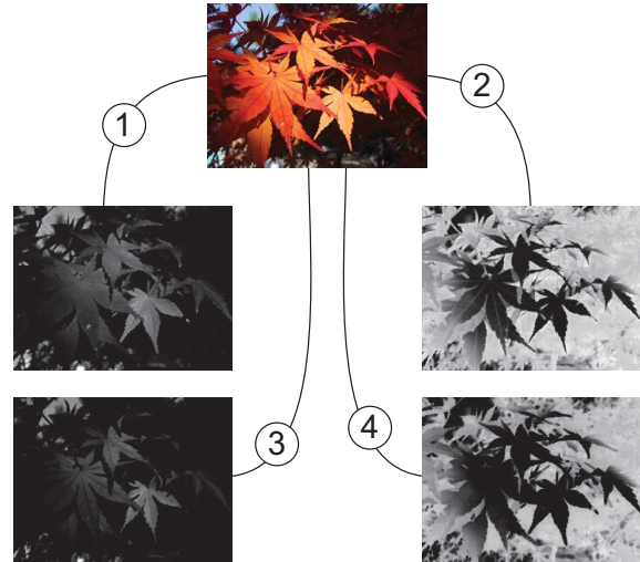
Figure 3. Application of the four hypervolume methods to a color image: 1 maximum union, 2 minimum union, 3 maximum section and 4 minimum section hypervolume.
